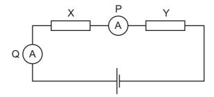
Which ammeter shows the current in resistor Y?
